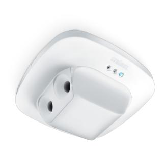
The US Hallway DCS is a digital (40kHz) ultrasonic technology occupancy sensor that utilizes STEINEL's stateof-the-art ultrasonic signal processing to provide superior stable volumetric bidirectional detection. The unique linear bidirectional coverage pattern is engineered specifically for hallways and applications requiring a true linear volumetric pattern of detection. This is an ideal hallway sensor for design and retrofit applications.
